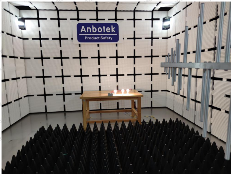
Photo of RF Field Strength Immunity Test
